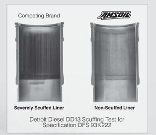
Based on third-party testing in the Detroit Diesel DD13 Scuffing Test for specification DFS 93K222.
