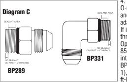
4. Lubricate the O-ring of the BP289 and install in the adapter assembly. If installing into the thread adapter (as in Option 2), tighten to 85 ft-lbs. If installing into the side of the BP402 (as in Option 1), tighten to 56 ft-lbs.
